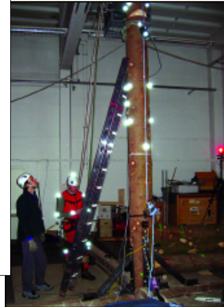
Figure 1. Stem and rigging set-up. Markers placed on the tree and the rigging system to track different motions (from top to bottom): the flight curve of the log, displacement and eventual slippage at the rigging point, deflection of the trunk, stretch in the rigging line.
