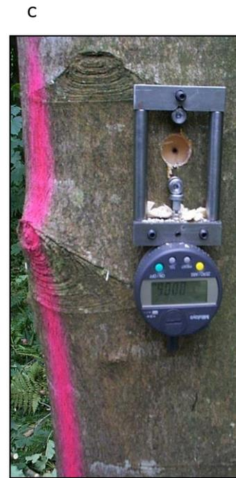
The CIRAD forêt growth gauge (DLRM) with a resolution of  $10^{-3}$  mm was used for stress measurements in a defined area.
