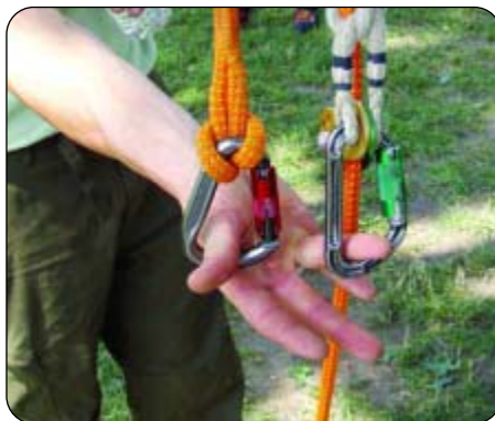
An example of a climbing system where two sides of the system are separated. Photo courtesy of Chris Cowell.
