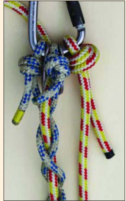
An example of multi-point wide loading of a carabiner. Photo courtesy of Chris Cowell.
