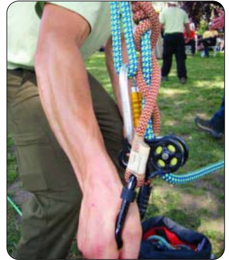
An example of a climbing system with a single point of attachment to the harness. Photo courtesy of Chris Cowell.
