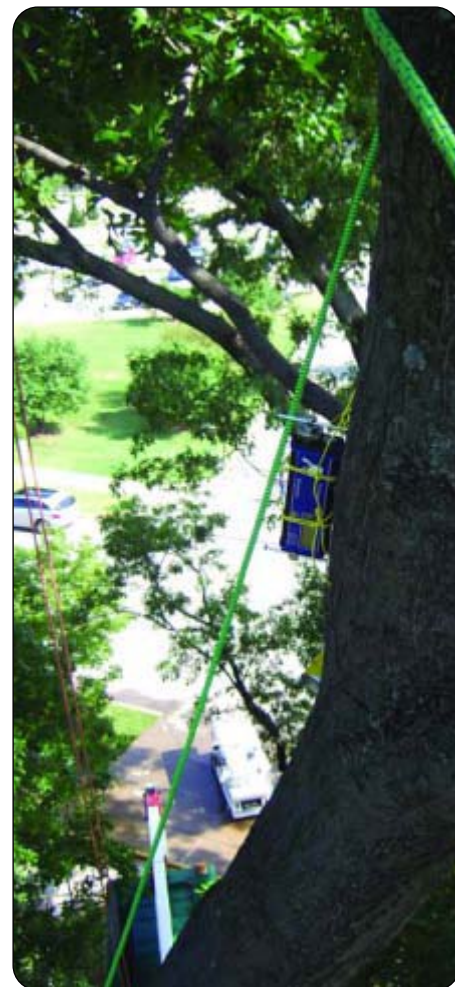
The TreeQinetic® strainmeter used to record a branch’s reaction when used as an anchor point. Photo courtesy of Andreas Detter.
