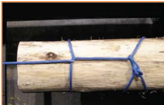
In the test lab, logs were fixed and the knots were set in a standardised manner. The ropes were pulled to failure and the peak forces were recorded.
