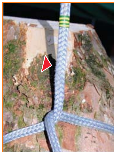
The yellow-green marker identifies the original position of the rope's point of entry to the half hitch. Note the visible abrasion of peripheral fibres on the left side of the rope after exiting the half hitch, indicating damage due to rope-to-rope friction under great load (red arrow head). The rope used was a 14mm double-braided PES line (Buccaneer Bullrope).
